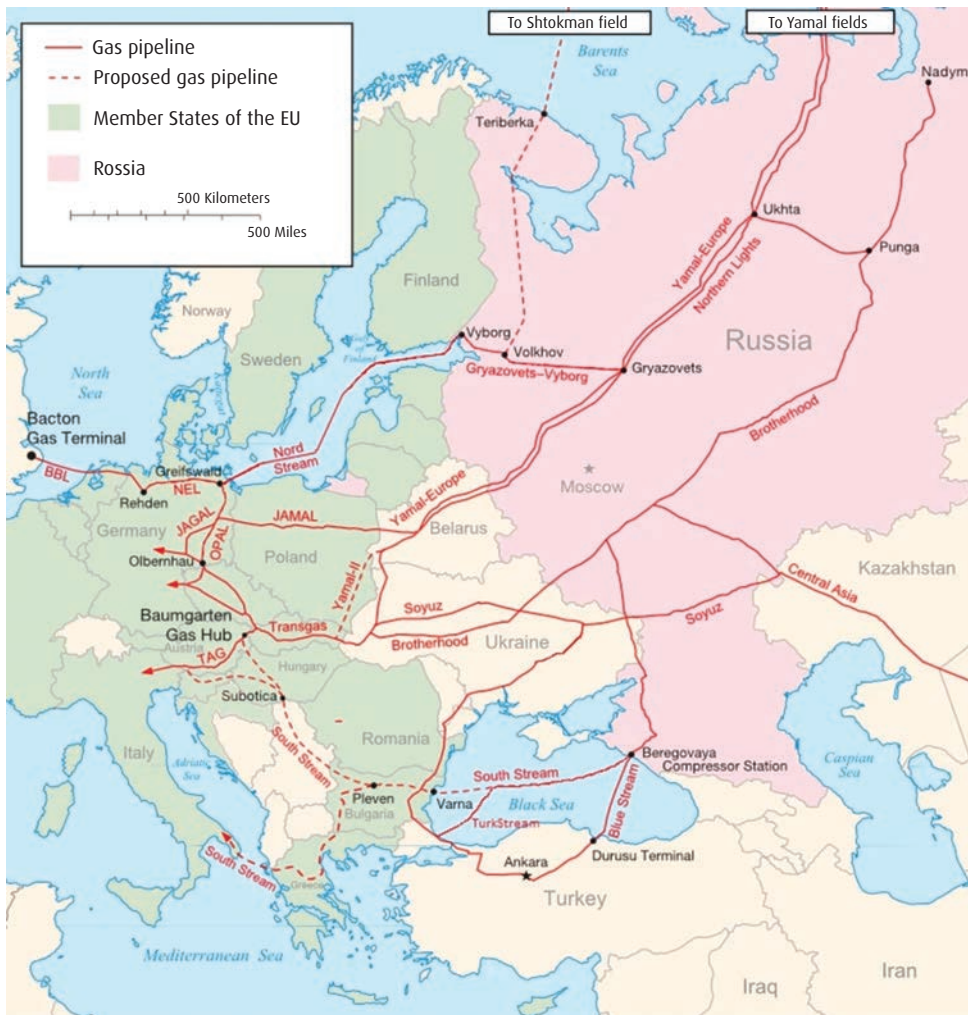
Figure 1. System of gas pipelines under construction and the existing ones
